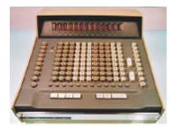
First electronic 4-function tabletop calculator ANITA MkVII. Its successor, the MkVIII, was the first successful commercial version. This (30 pounds) product of the British firm Sumlock Comptometer and Bell Punch, used 177 gas-filled thyratron tubes as switching elements. Internally however, this calculator operated still on a decimal basis, not digital. The keyboard still looked like a "Comptometer".
