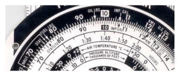
An aircraft's altitude is determined by measuring the pressure of the outside air using a special type of barometer (static pressure). Altimeters are calibrated according to a standard atmosphere that has a temperature of 15° C at sea level and a well-defined pressure and temperature gradient.
