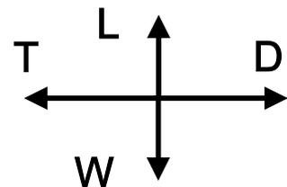
Lift is generated by the movement of air over the (curved) wing surface, and it is the combination of air speed, angle of incidence (the angle between the wing and the air stream) and parameters determined by the wing profile used, that determine how much lift is generated and where its center of lift is located along the wing cord. Now, how do we control the center of lift to cater for a changing center of gravity (like that passenger moving along)? In fact,
