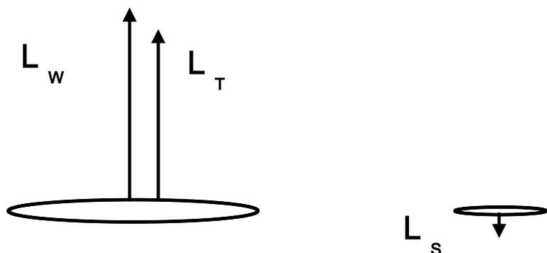
the picture is slightly more complicated. Total lift **L<sub>T</sub>** is a vector resulting from the addition of two separate lift vectors: a positive one (upward) on the wing **L<sub>W</sub>** and a negative one (downward) on the horizontal stabilizer **L<sub>S</sub>**.
