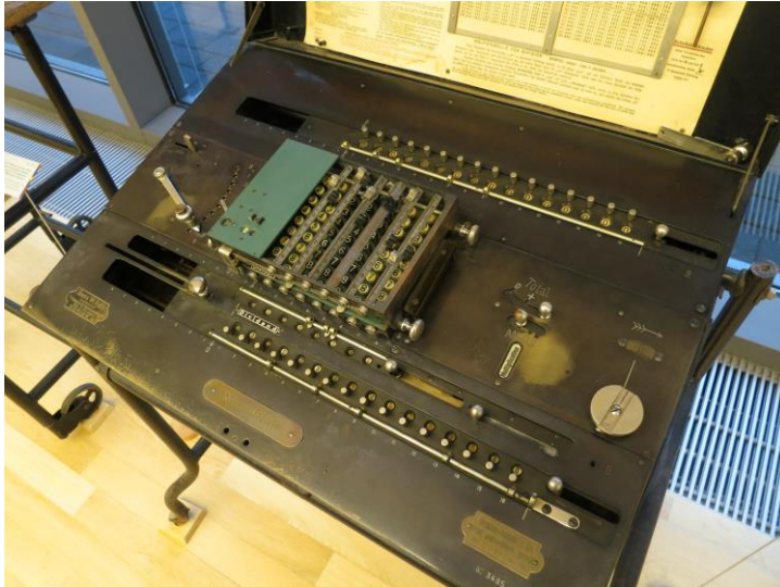
Figure 14. Motorized Millionaire with keyboard, constant mechanism and second total counter, on a custom made table
