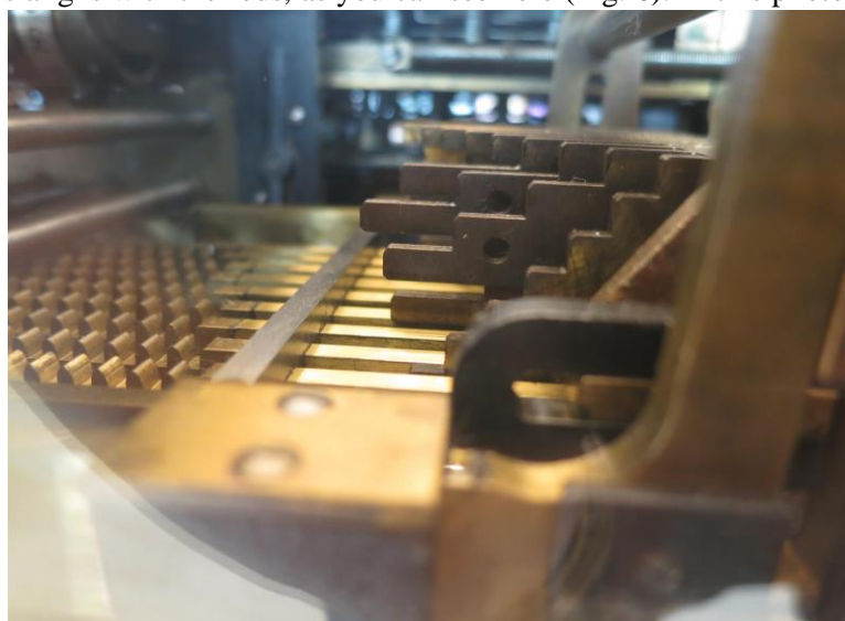
Figure 6. The ein-mal-eins in position for the table of seven
